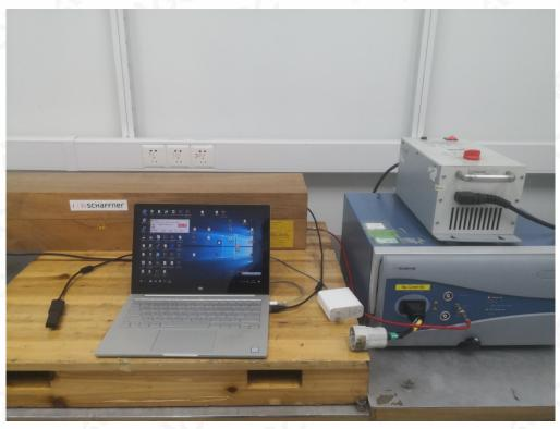
EN 61000-4-6 CS IMMUNITY TEST SETUP-AC POWER PORT
