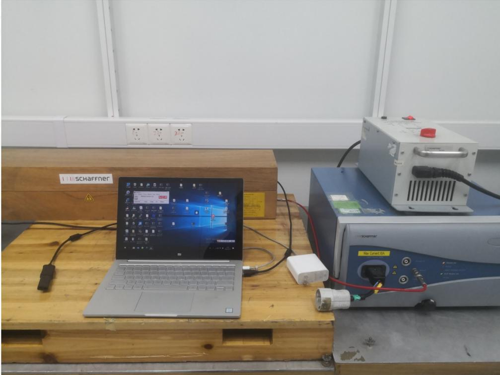
EN 61000-4-6 CS IMMUNITY TEST SETUP-AC POWER PORT
