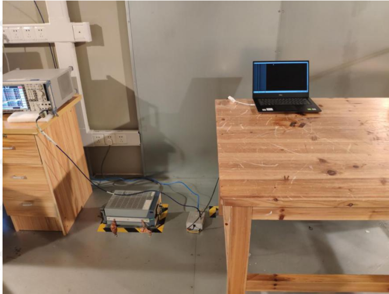
Photograph of test setup for Conducted Emission
